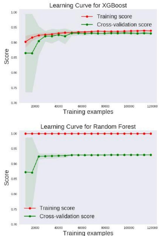
Figure 4: Learning curves for `XGBoostClassifier` and `RandomForestClassifier`. Note the gap between the training and cross-validation scores for the Random Forest Classifier. A persistent gap combined with a perfect or near-perfect learning score is an indicator of overfitting.
